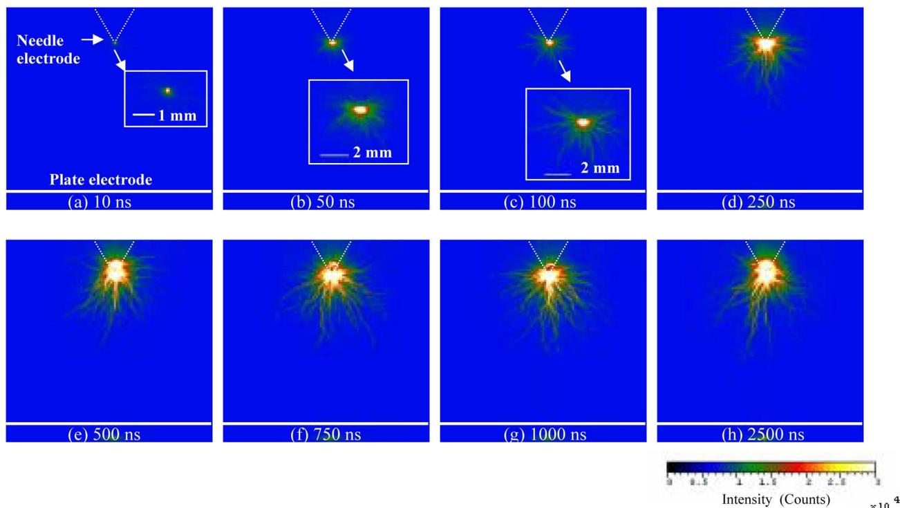
Fig. 2. Accumulated images of 20 streamers in distilled water (applied voltage: 27 kV; discharge current: 4–6 A; and gap: 20 mm). Each image is plotted with the same intensity scale: (a) 10 ns; (b) 50 ns; (c) 100 ns; (d) 250 ns; (e) 500 ns; (f) 750 ns; (g) 1000 ns; and (h) 2500 ns.
