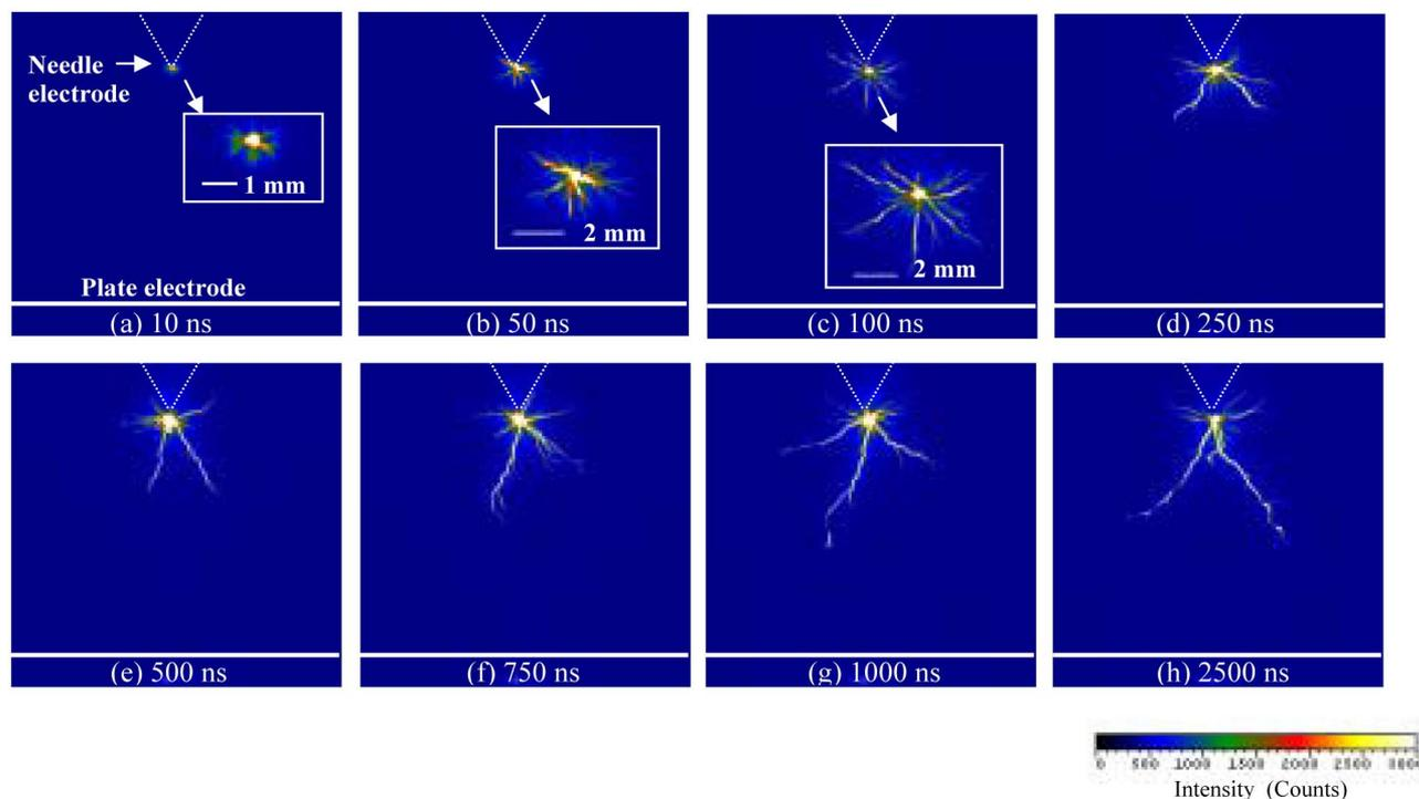
Fig. 1. Time evolution of pulsed streamers generated by a single discharge in distilled water (applied voltage: 27 kV; discharge current: 4–6 A; and gap: 20 mm). Each image is plotted with the same intensity scale: (a) 10 ns; (b) 50 ns; (c) 100 ns; (d) 250 ns; (e) 500 ns; (f) 750 ns; (g) 1000 ns; and (h) 2500 ns.
