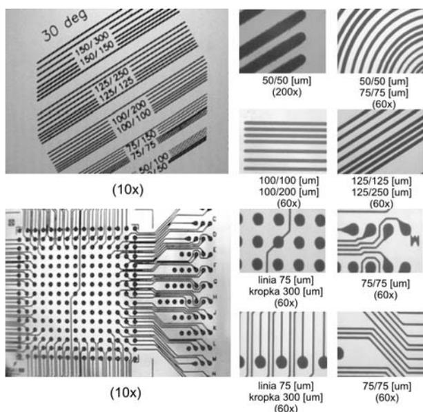
Fig. 4. "Lines" and "BGA" patterns on PCB after etching process
