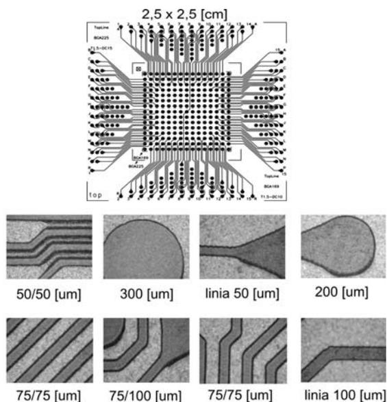
Fig. 3. Pattern BGA (Ball Grid Array) and tracks on photoresist
