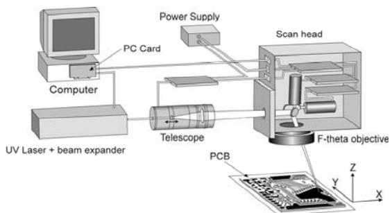
Fig. 1. Schema of LDI system connections [4]
