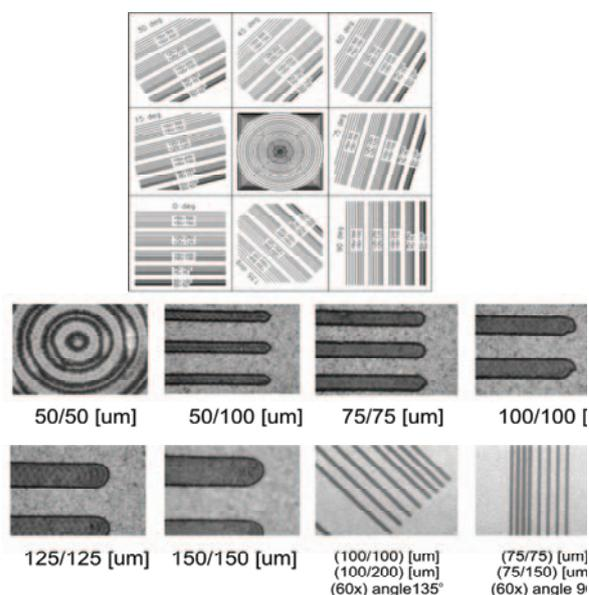
Fig. 2. Test pattern consisted of lines with different widths and angles and also circles inside
