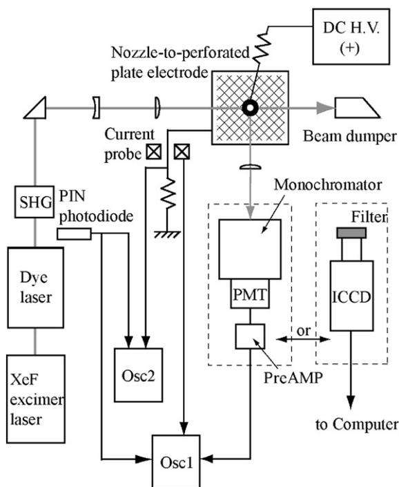
Fig. 1. Schematic diagram of the experimental apparatus (top view).
