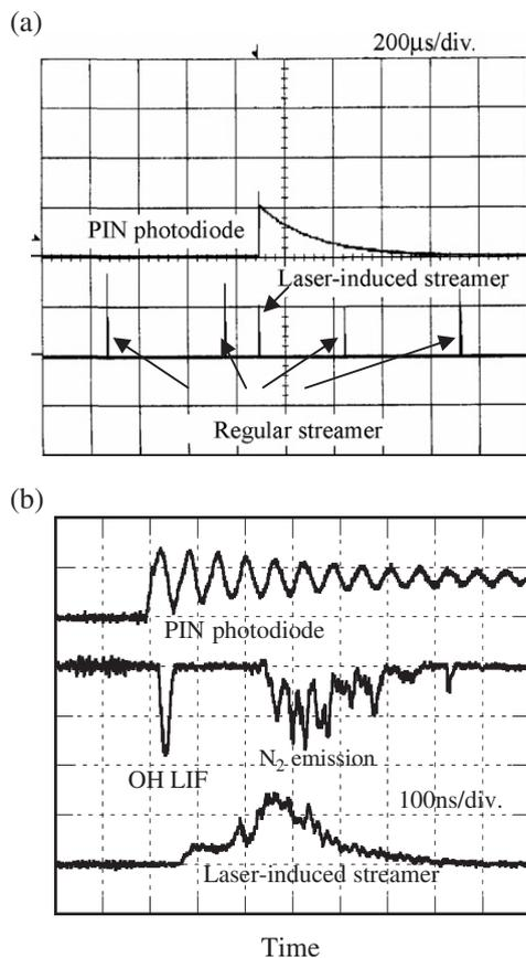
Fig. 3. Timing relationship between laser detected by a PIN photodiode, OH LIF signal and current waveform of laser-induced streamer. The applied voltage is 29 kV and corona current is 185 μA. (a) Regular streamer current pulses and laser-induced current pulse. (b) Typical waveforms of OH LIF signal and laser-induced current pulse. The peak current of laser-induced streamer is 90 mA.
