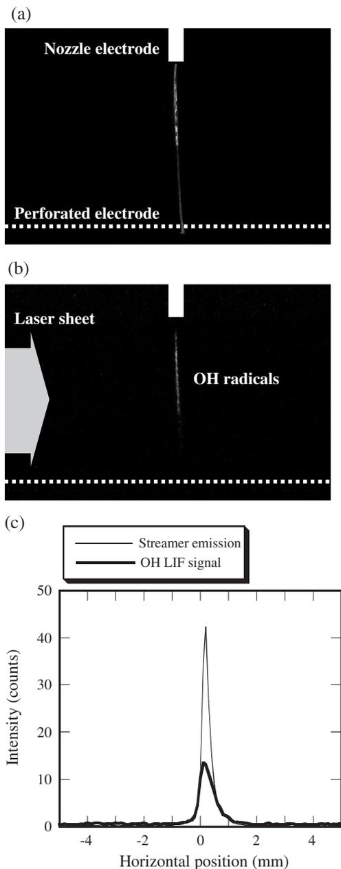
Fig. 6. Comparison of streamer and LIF images in open air. The applied voltage is 14 kV and corona current is 60  $\mu$ A. (a) streamer emission observed by the ICCD camera with gate time of 900  $\mu$ s; (b) OH LIF between the electrodes (ICCD gate of 100 ns); (c) horizontal profile for both streamer emission and OH LIF.
