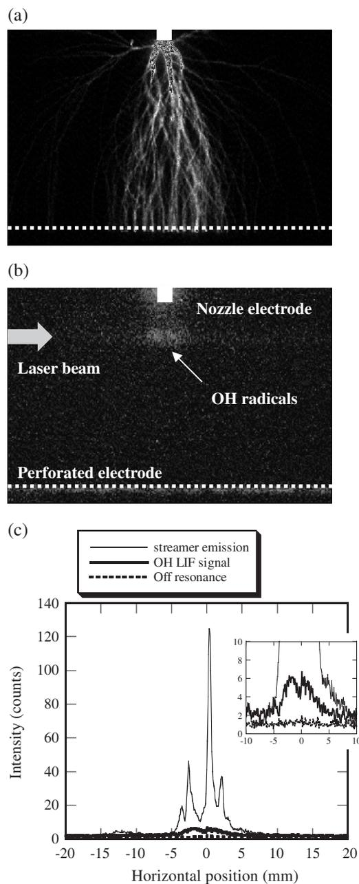
Fig. 5. Comparison of streamer and LIF images in open air. The applied voltage is 29 kV and corona current is  $190 \mu\text{A}$ . (a) streamer emission observed by the ICCD camera with gate time of  $900 \mu\text{s}$ ; (b) OH LIF near the tip of the stressed electrode (ICCD gate of  $100 \text{ns}$ ); (c) horizontal profile for both streamer emission and OH LIF. The profile obtained at the laser wavelength of off-resonance is also shown.
