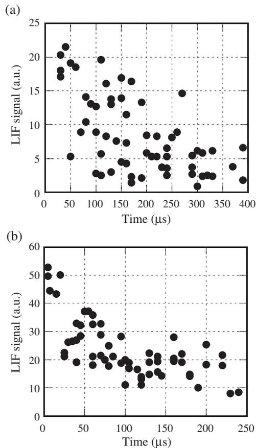
Fig. 4. Time evolution of OH LIF signal after the last streamer before the laser incidence: (a) in open air without Ar gas flow (applied voltage 29 kV, corona current 200 μA); (b) in open air with Ar gas flow (applied voltage 11 kV, corona current 40 μA).
