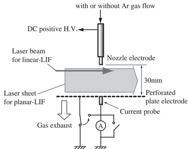
Fig. 2. Schematic diagram of the discharging region and incident laser for LIF measurement (side view).
